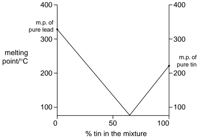
The graph shows that any mixture of lead and tin must have a melting point
